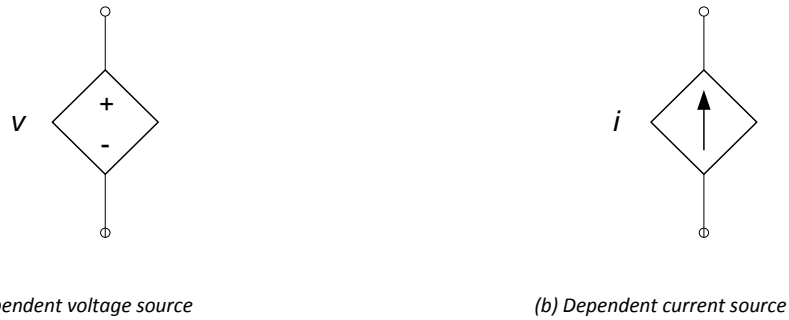
Figure 1.5. Symbols for dependent sources.
