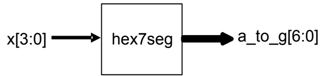
Figure 9.3 A hex to 7-segment decoder
